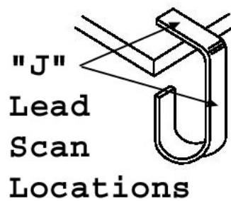
FIGURE 2037-3. Scan Locations on J-Style lead.
